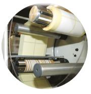
The **Uranus** is non-stop 2 spindle turret rewinder with automatic glue system, auto eject of the rewound cores, and fast mandrel change system. Suitable to fit behind a wide range of roll to roll labels converting and printing presses with a simple electrical interface and no mechanical connections. Easy handling, easy to carry, reliable and economic non-stop rewinder. Can add slitting as options.
