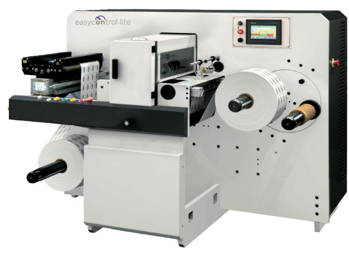
The **Easy control** lite automatic slitter rewinder is fully servo-driven and features taper tension control, web guide, a turret rewinder, meter and number of labels counting, static eliminator etc.
