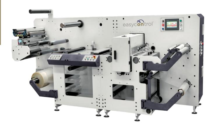
The **easy control** is a fully servo advanced inspection slitter rewinder with excellent tension control suitable for label stock and thin film material.
