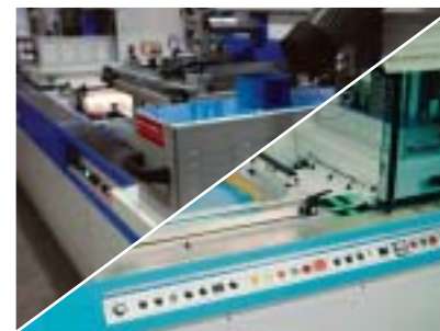
▲ Removable UV drying cassette. 120 Watts / cm with double air exhaust system (160 watts in option).
