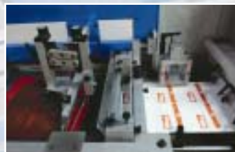
Registration perforator on the first group (for registration of other printing stations and finishing and converting units).
