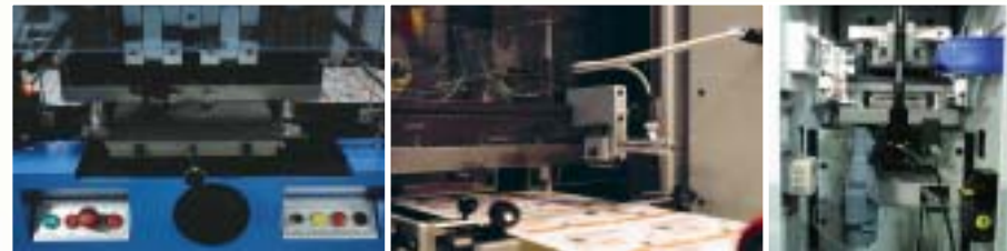
Traditional steel rules dies or magnetic dies can be used (optional).
