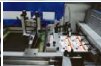
Registration cell located in front or behind the screen according to the number of passes.
