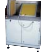
▲ Cleaning fountain. Ideal to clean at the exit of the machine screens, squeegees and flood bars.
