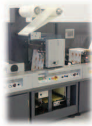
Station flexo UV. Pelliculage (option). Chariot mode semi-rotatif (option). UV flexo station. Laminating station (option). Semi-rotary mode trolley (option).
