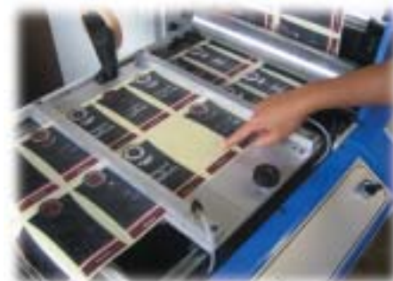
Automatic stop at the second splicing table in case of default.
